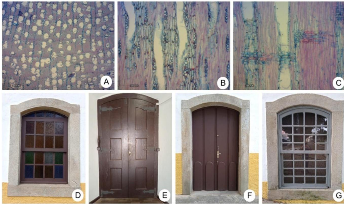
Figure 12. Constructive element and respective wood anatomy of Handroanthus sp. (Bignoniaceae), Nossa Senhora da Graça Church, São Francisco do Sul, Santa Catarina State, Southern Brazil. Caption: (A) Transverse section. (B) Radial longitudinal section. (C) Tangential longitudinal section. (D – G) Frames present in the building
