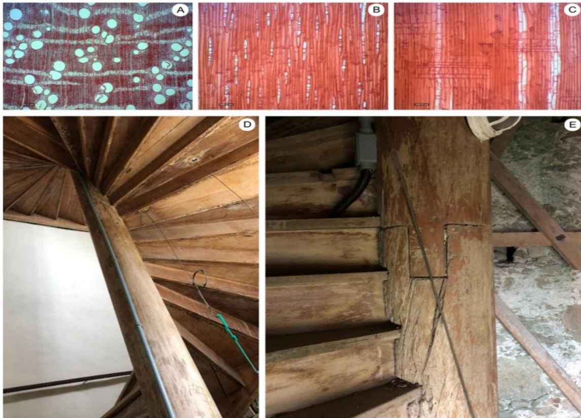
Figure 6. Constructive element and respective wood anatomy of Calophyllum brasiliense (Calophyllaceae), NossaSenhora da Graça Church, São Francisco do Sul, Santa Catarina State, Southern Brazil. Caption: (A) Transverse section. (B) Radial longitudinal section. (C) Tangential longitudinal section. (D–E) Pillar of the bell tower structure.
