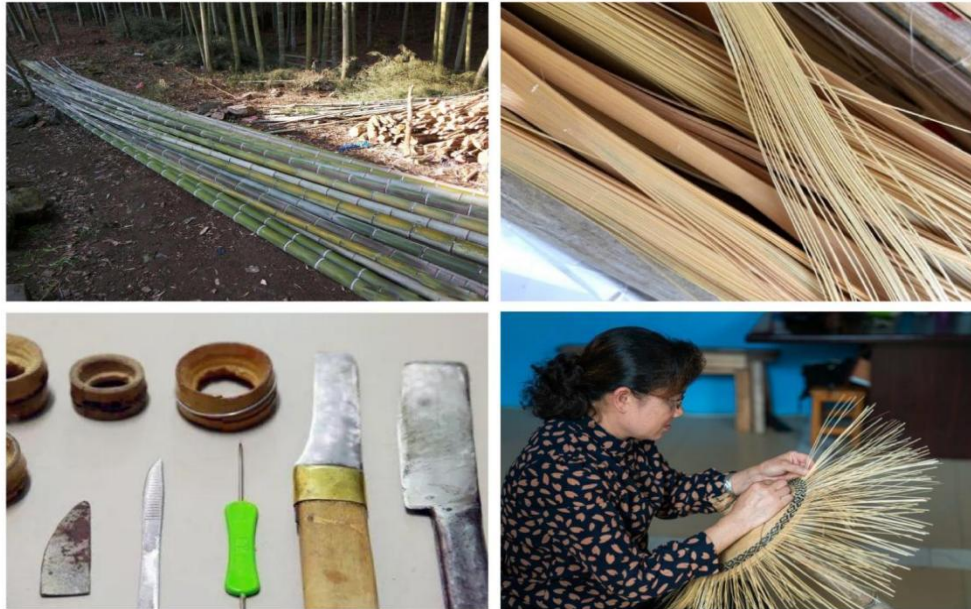
Figure 1 - Materials and weaving tools of Maonan flower bamboo hat
